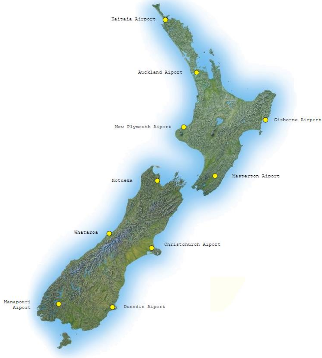
Figure 5: Transpower's lightning detection network
